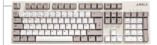
Multimedia function shortcuts can accessed by holding the right *A* key and pressing F1 to F12. (Assuming key positions match the default PC layout pictured above. The Alt and *A* key positions can be swapped and remapped in order to achieve a legacy Amiga layout if required.)
